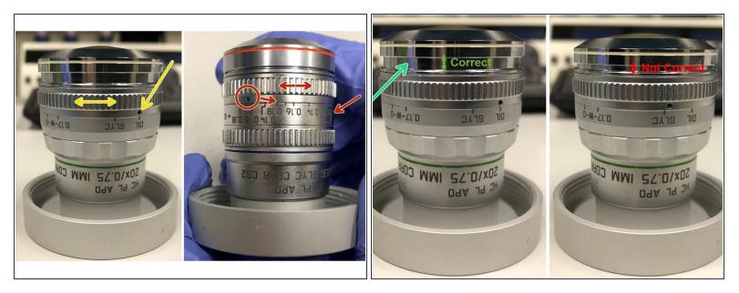
A For some objectives the **correction collar** has to be adjusted.
