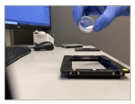
Insert the 35 mm Petri dish into the KM Frame.
