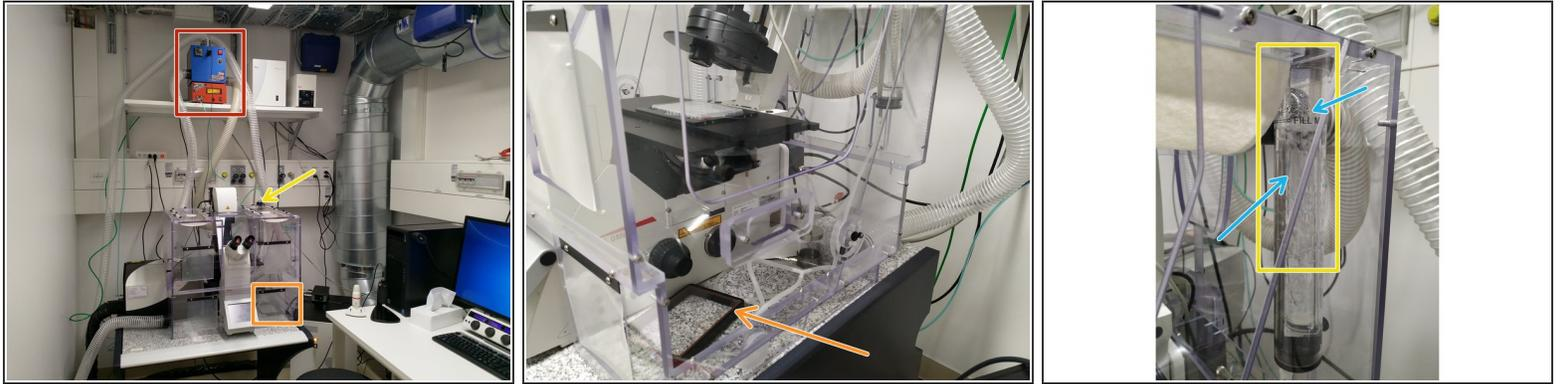
**i** **Start heating** at least 30 min before you start your experiment. This allows the chamber and the microscope components to heat up and avoids drift during your experiment.
