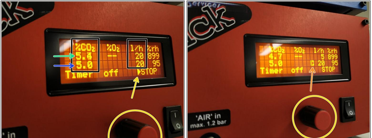
**i** After turning on, the gas flow should start automatically.
