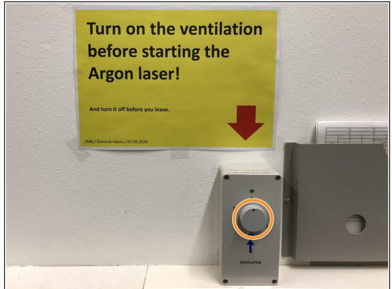
**⚠ Engaging the argon laser without turning on the ventilation/cooling will lead to thermal destruction.**
