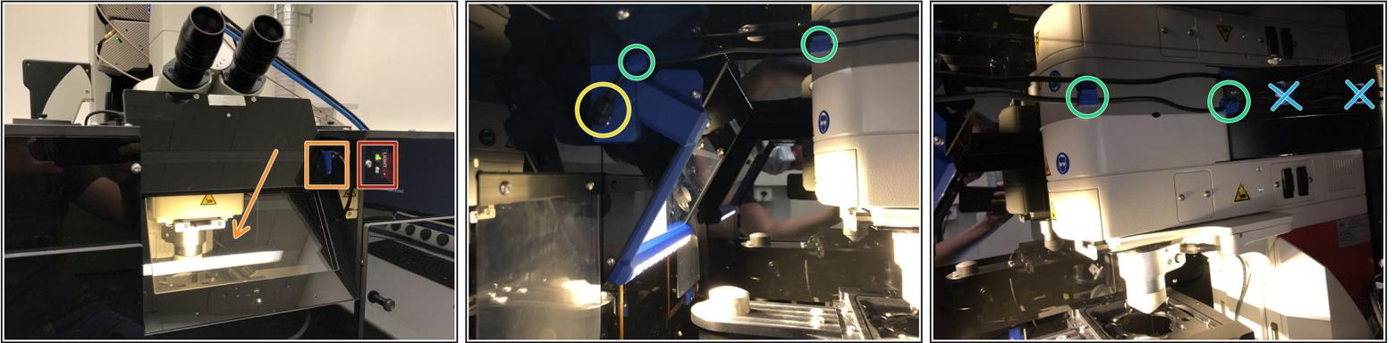
**i** Due to the new detector geometry, the microscope is outfitted with a new light insulation box. Only remove the front part of the box when absolutely needed.
