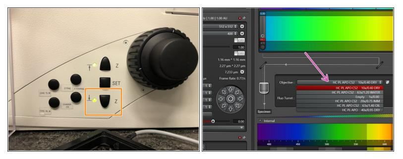
Lower the objective turret by pressing the "Z" downwards button on the right side of the microscope.
