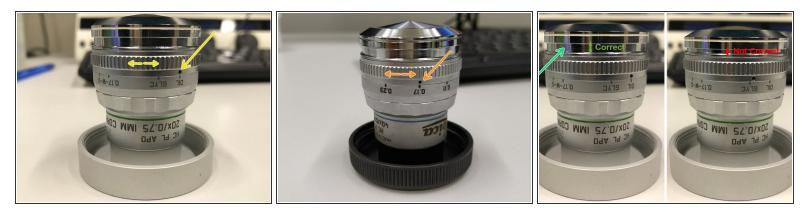
A For optimal imaging performance on some objectives the **correction collar** has to be adjusted.
