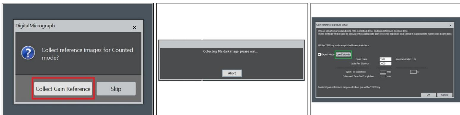
**⚠ For the Gain reference in counting mode, you need a much lower electron dose!!!! Bring the screen down and increase the spot size to 4 or 5, before starting. Then you can lift the screen again.**
