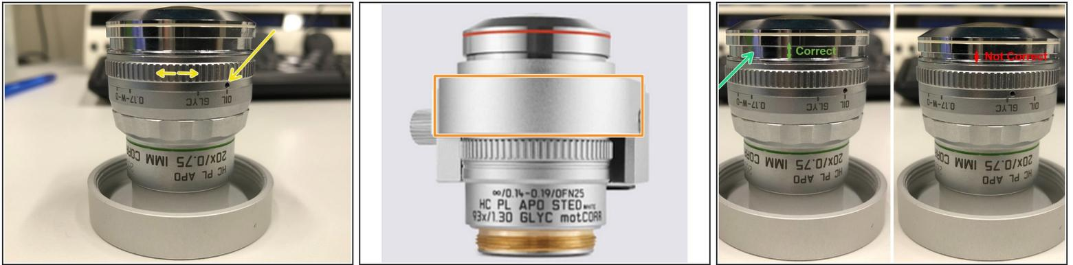
**⚠** For optimal imaging performance on some objectives the **correction collar** has to be adjusted:
